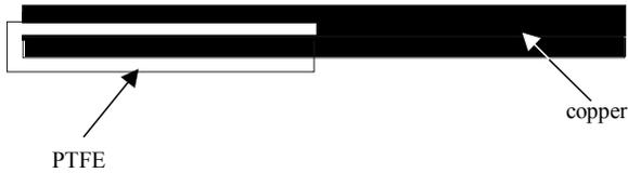
Figure 2: Flat rod section (sketch)
