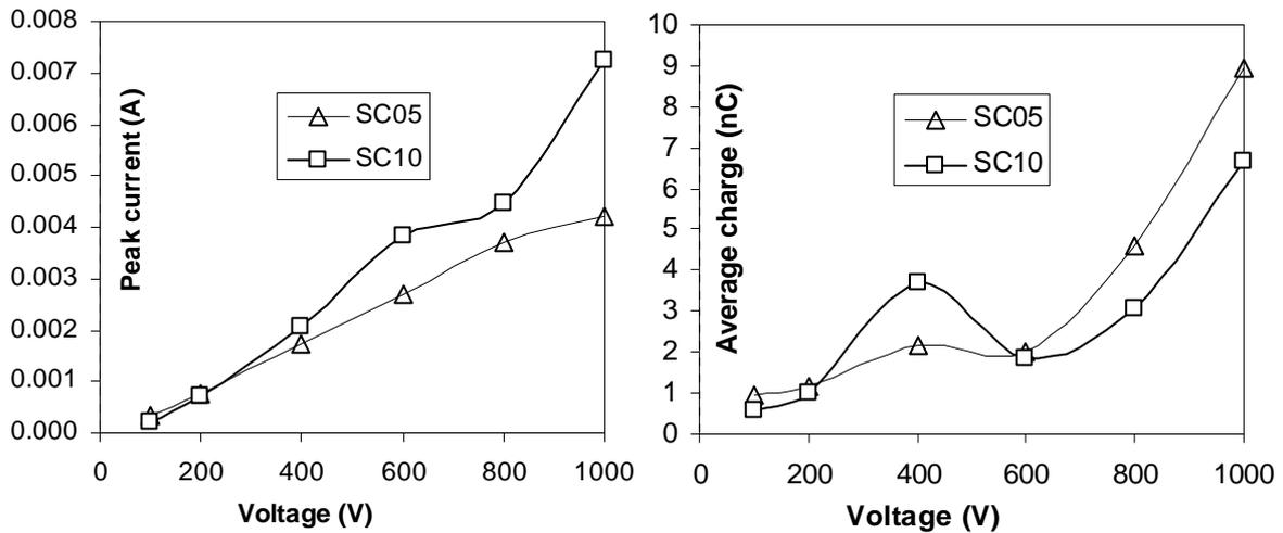
Figure 3. a) Average peak discharge current and b) average charge from a discharge as function of the charging voltage for the SC05 and SC10 fabrics.
