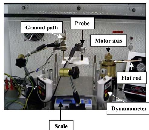
Figure 1: A view of the test cell
