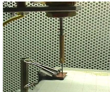
Fig. 2: Electrode grounded by a needle
